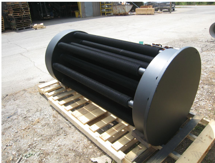
Photos of one of the Blue Smoke Condenser to be installed at FMCC Plant 1
