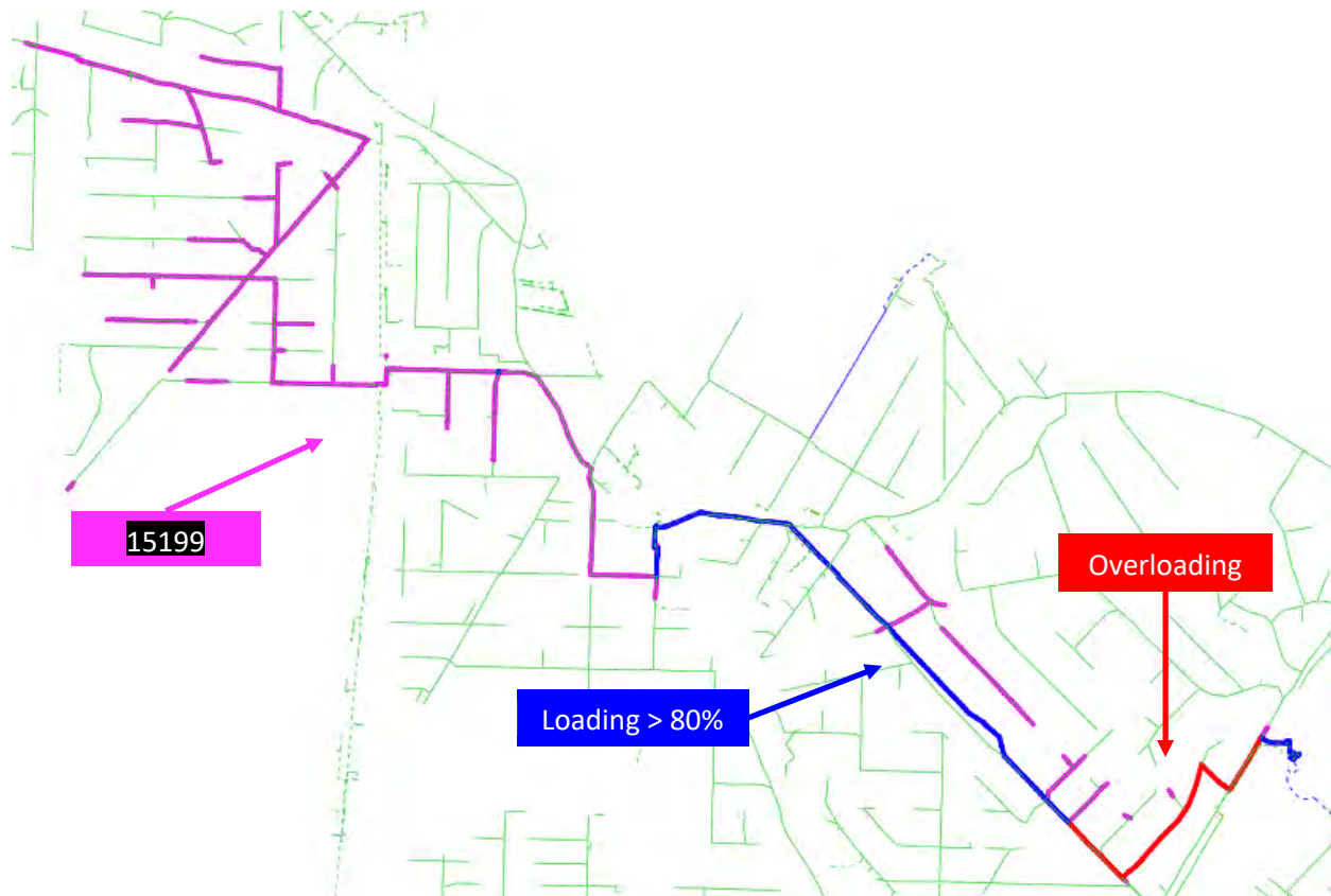
Figure A.23: Loading violation of Feeder 15199 under normal condition in 2032 with electrification and EV impact
