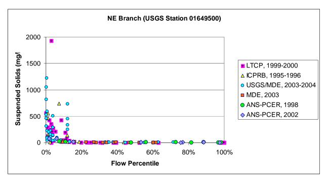
Figure 8. Suspended Solids Data for NEB, 1995-2004, versus Flow Percentile
