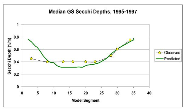
Figure 13. 1995-1997 median growing season Secchi depth in tidal Anacostia River: predicted by calibrated model vs. observed
