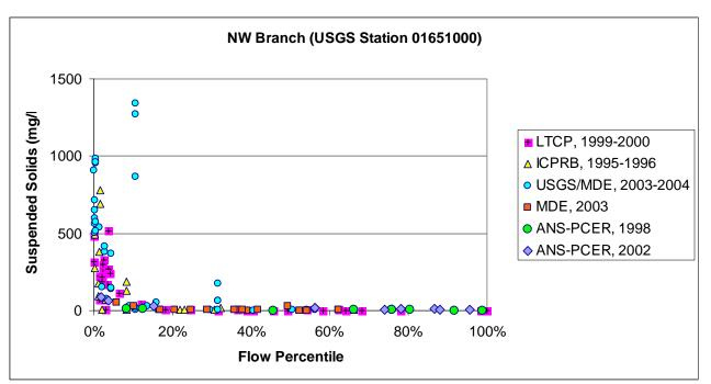
Figure 9. Suspended Solids Data for NWB, 1995-2004, versus Flow Percentile
