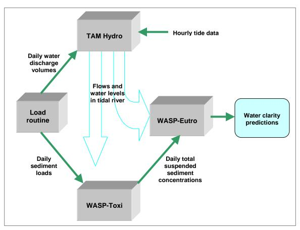
Figure 12. Schematic diagram of TAM/WASP modeling framework
