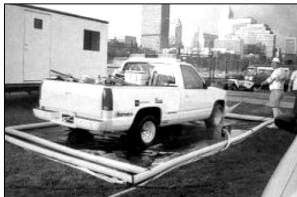
EPA's National Compliance Assistance Center's: http://www.epa.gov/nca Preventing Wash Water from Entering the Storm Drain
