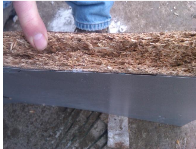
View of particleboard found during systems furniture deconstruction.
