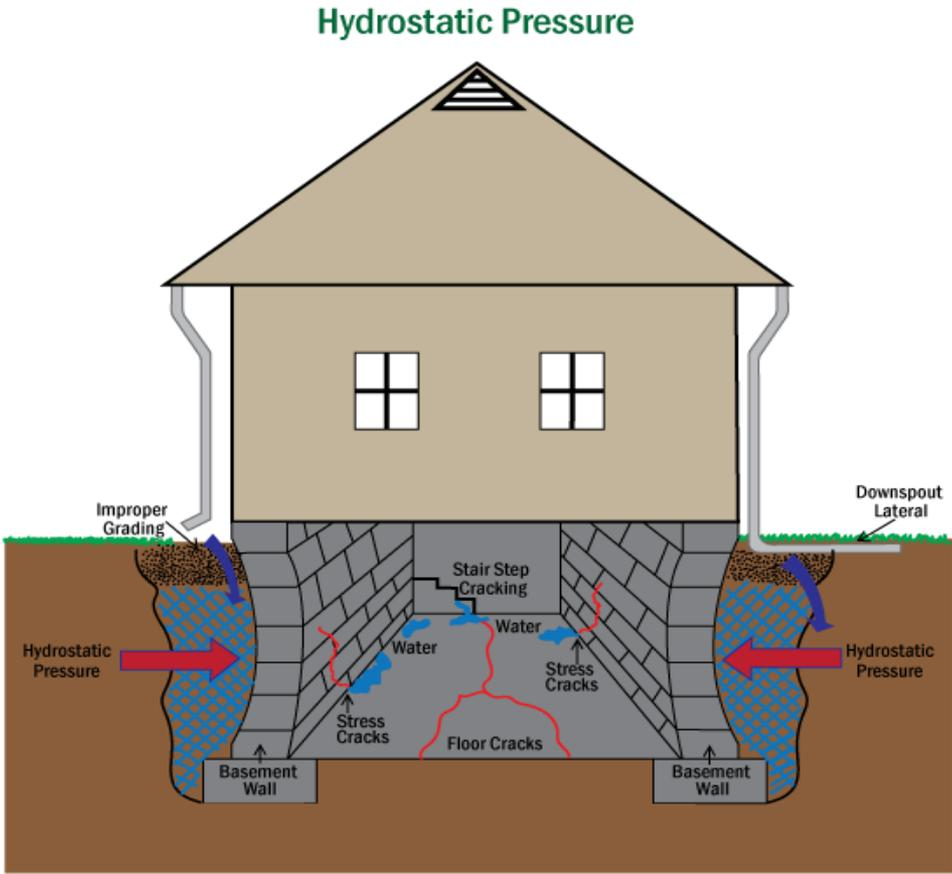
Collapse of basement and structural damage to foundation.
