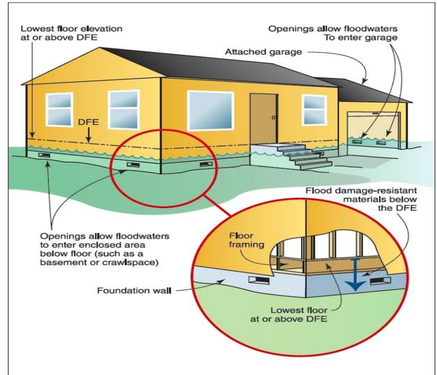
Wet floodproofing - Flood-damage-resistant materials **minimize flood damage** to areas **below the flood protection level** of a structure, which is intentionally allowed to flood.
