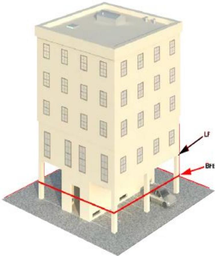
Elevated on piers with wet-floodproofed stairwell.
