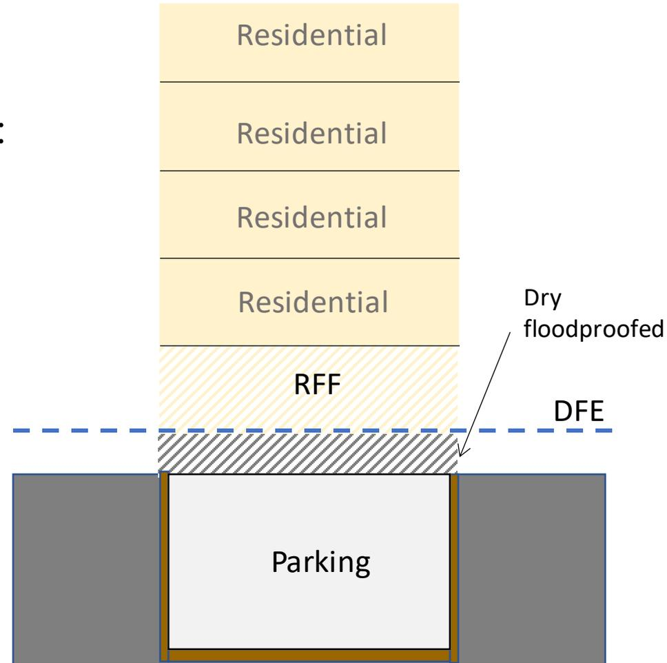
Basement is watertight and reinforced to withstand flood loads specified in ASCE 24-14
