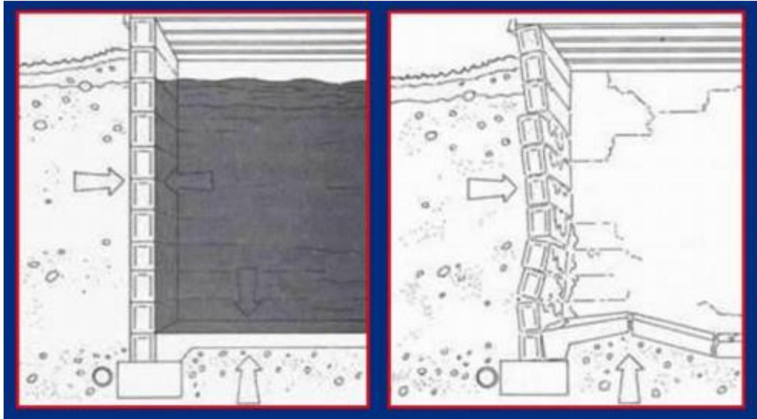
Dry-floodproofed basements are engineered to withstand external forces and prevent collapse.
