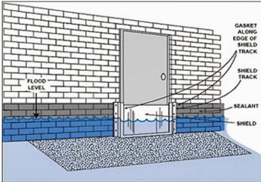
Dry floodproofing - Structure, including the attendant utilities and equipment, is **watertight** with all elements substantially impermeable to floodwater and with structural components having the capacity to **resist flood loads**.
