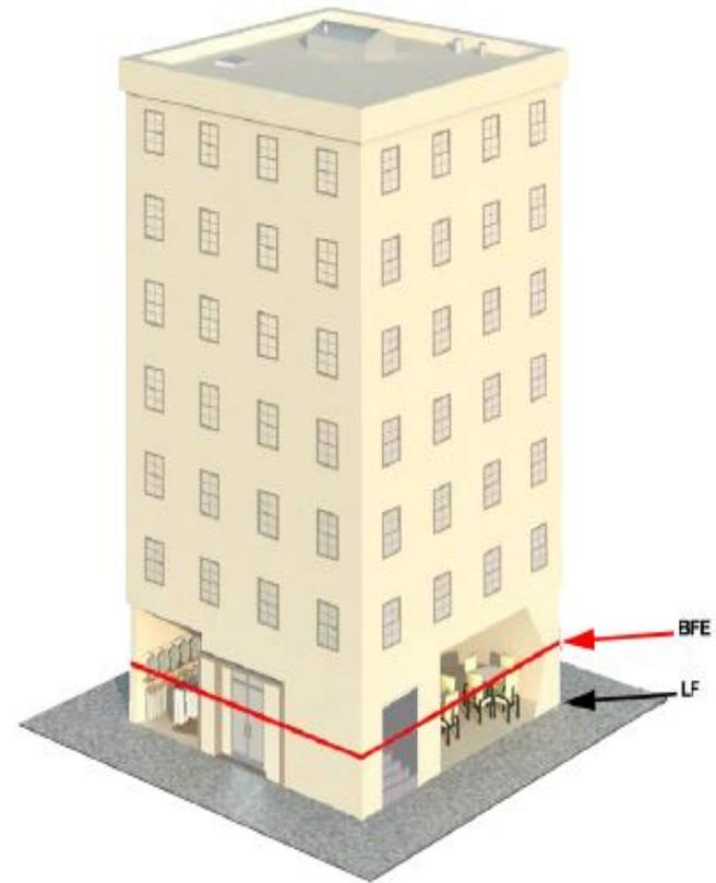
Commercial uses (laundry service and restaurant) are located below DFE but dry-floodproofed. Note separate wet-floodproofed building access for the residential spaces.
