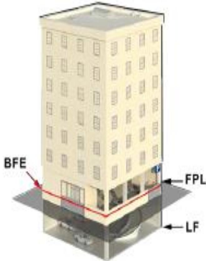
Note deployed flood shield at entrance. Underground parking for mixed-use buildings currently (June 2021) requires an approved code modification, but will be allowed by-right under proposed Regulations
