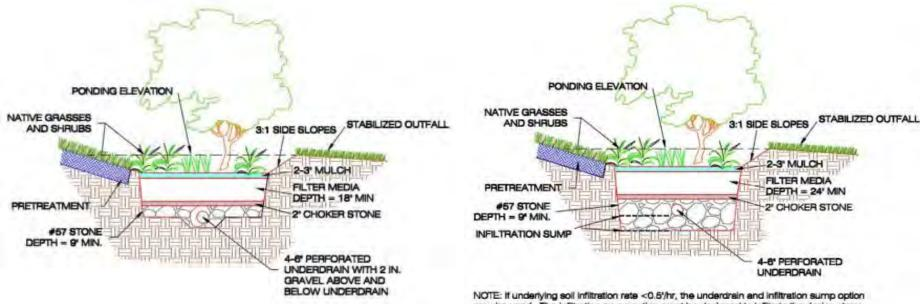
may be used. The infiltration sump option must be designed to infiltrate the design storm volume in less than 72 hours.
