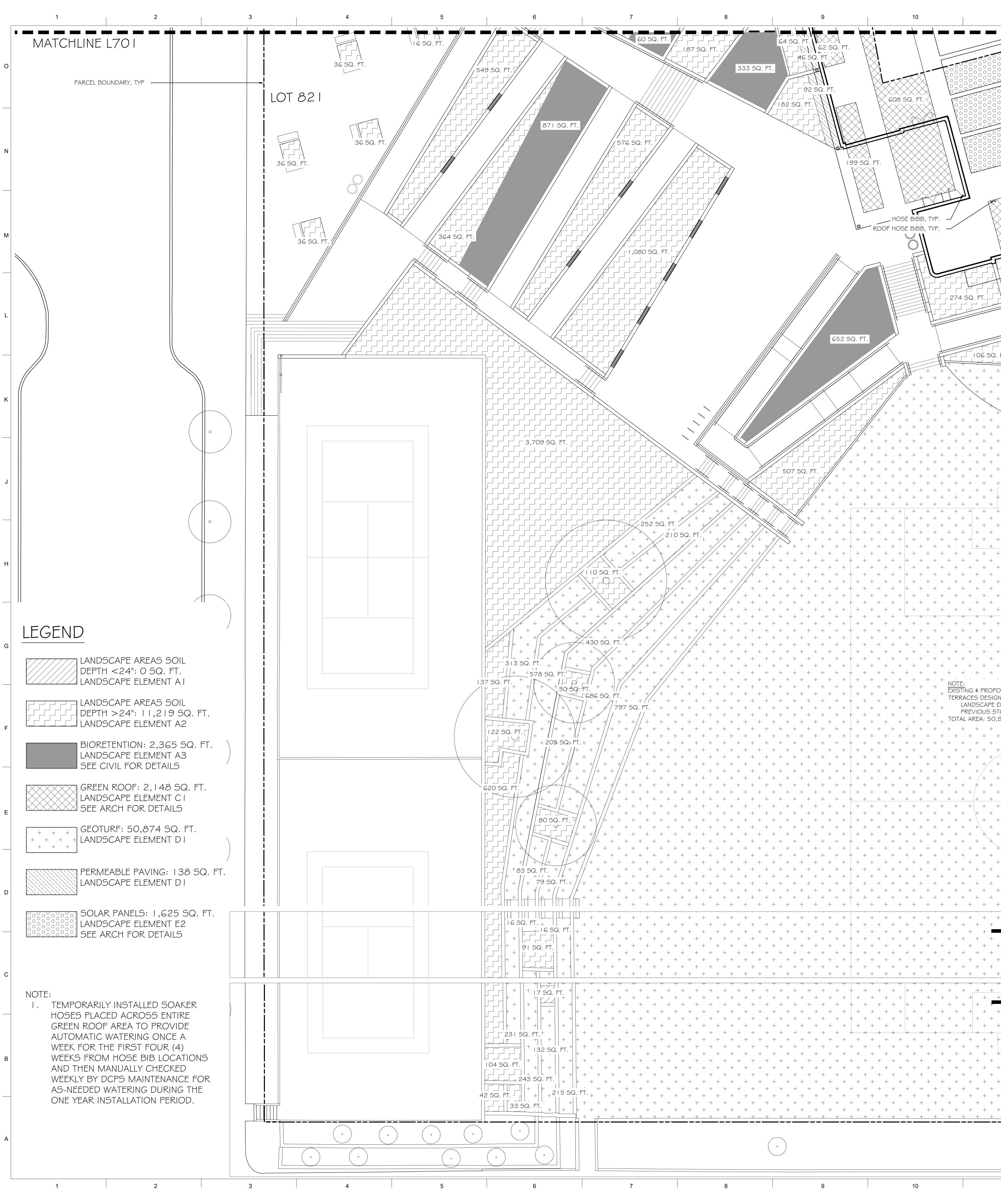
13 62 SQ. FT. 365 SQ.  $\times \times >$ 594 SQ. FT I = X / I608 SQ. FT. 594 SQ. FT 199 SQ. FT.  $\times$   $\times$   $\land$ HOSE BIBB, TYP. ROOF HOSE BIBB, TYP. 209 SQ. FT 274 SQ. 250 SQ. F1 652 SQ. FT. 449 SQ. FT. 106 SQ. FT EXISTING & PROPOSED SYNTHETIC TURF SOCCER FIELD (46,291 SQ. F FERRACES DESIGNED AS PERMEABLE PAVING (4,649 SQ. FT.) LANDSCAPE ELEMENT D I PREVIOUS STORMWATER MANAGEMENT APPROVAL - #3603 TAL AREA: 50,940 SQ. FT. <sup>\_\_</sup> 203 SQ. FT. 11 13
