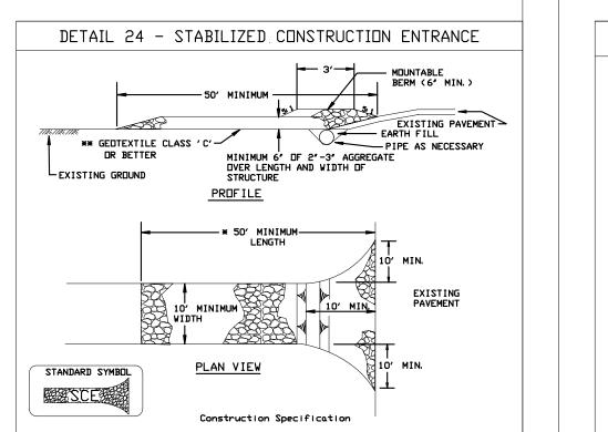
1. Length - minimum of 50' (\*30' for single residence lot). 2. Width - 10' minimum, should be flared at the existing road to provide a turning radius.
