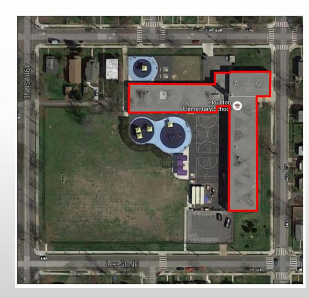
$SWRv(cf) = \frac{P}{12 in/ft} \times [0.95 \times (Impervious Area) + 0.25 \times (Compacted Area)]$
