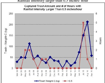
Figure 5-3-6: Captured Trash Amount and Number of Hours with Rainfall Intensity larger than 0.5 inches/hour
