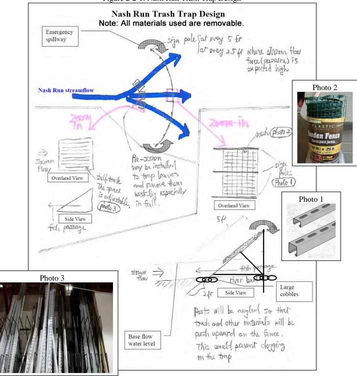
Figure 2-2-1: Nash Run Trash Trap Design
