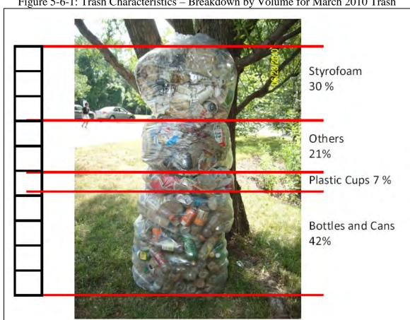
Figure 5-6-1: Trash Characteristics – Breakdown by Volume for March 2010 Trash
