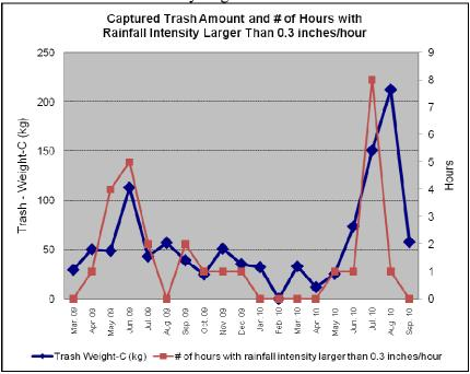
Figure 5-3-5: Captured Trash Amount and Number of Hours with Rainfall Intensity larger than 0.4 inches/ hour
