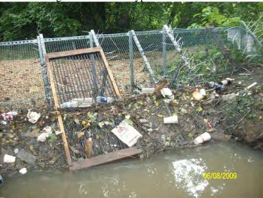
A prototype re-bar screen was placed on top of the plastic net to see what kinds of trash could be captured and what kinds escape. Other types of screens (bamboo and fishing wire) were also tested but proven ineffective.
