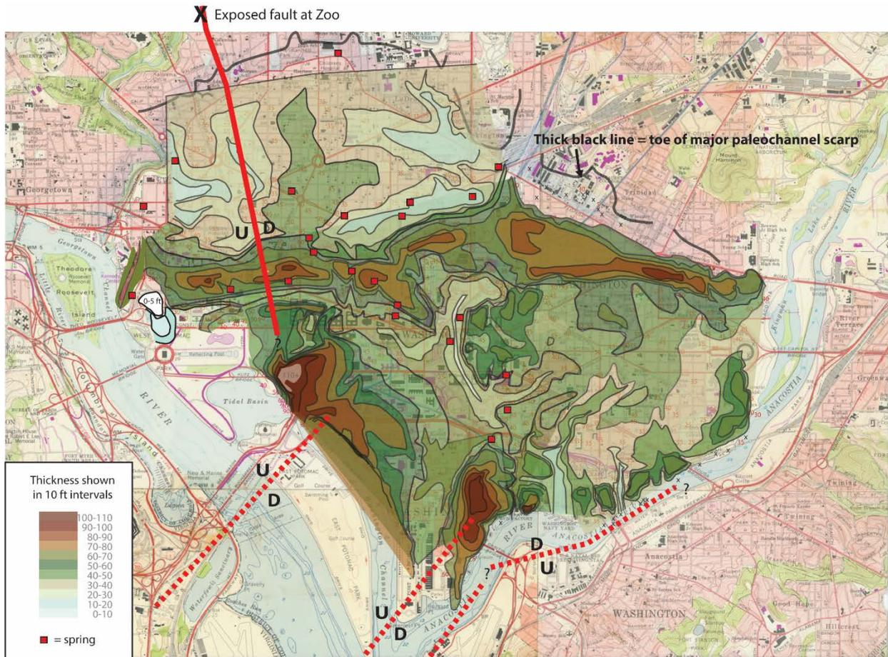
**Figure 5.2** Map of the thickness of the Quaternary deposits beneath downtown Washington D.C. Thicker areas are sandy infillings of paleochannels and are groundwater reservoirs and conduits. The locations of most springs coincide with steep gradients where younger channel erosion cuts into older paleochannel deposits.
