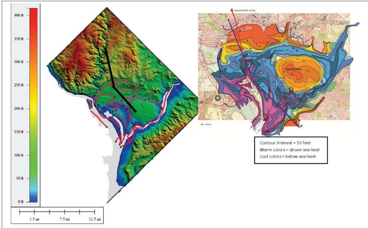
**Figure 5.1 (Left) LiDAR elevation map of Washington D.C. and the paleochannels found in the current joint USGS-DOEE study (arrows pointing downriver). (Right) Structure contour map of base of Quaternary sediments showing numerous paleochannels and locations of proposed faults (red dashed lines) and documented fault (solid red line).**
