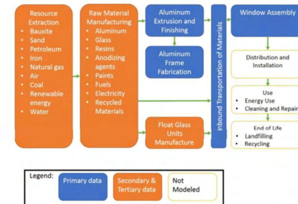
Figure 1: Life cycle stage diagram for cradle-to-gate production of traditional curtain wall by Kawneer
