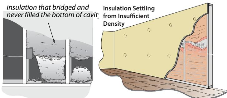
**Problems with low density insulation:** Blowing insulation through one or two small holes usually creates voids inside the wall cavity. This is because insulation won't reliably blow at an adequate density more than about one foot from the nozzle. Use tube-filling methods whenever possible, using a 1.5-inch hose inserted through a 2-inch or larger hole.
