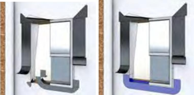
**Flashing nail-fin windows:** Installers place the window on and over the sill flashing. The side and top flashing cover the fastening fin. The two methods shown here are: using a flexible membrane (right) and using a bow-tie-shaped flashing to underlay the corners when using a standard membrane.
