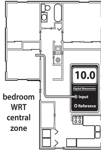
**Pressurized bedrooms:** Bedrooms with supply registers but no return register are pressurized when the air handler is on and the doors are closed. Pressures this high can double or triple air leakage through the building envelope.
