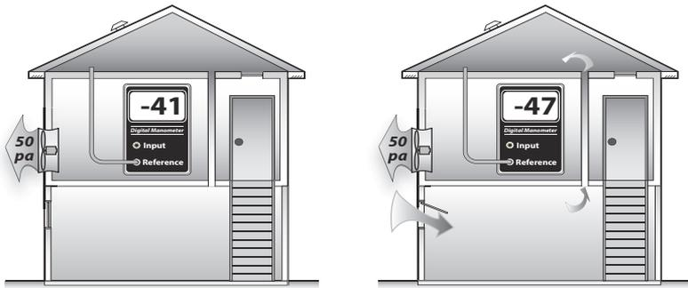
**Zone connectedness:** The attic measures closer to outdoors after the basement window is opened, indicating that the attic and basement are connected by a large bypass.
