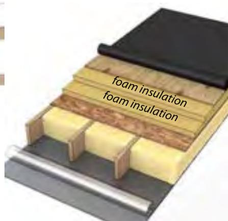
**Rooftop foam insulation:** The IRC code requires foam insulation over the structural sheathing when the roof is unventilated.
