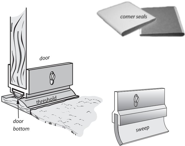
**Weatherstripping at the door bottom:** A threshold and door bottom are the ideal bottom seal for a door. The threshold and door bottom must be adjusted to seal but not bind. Corner seals in the bottom complete a quality door-weatherstripping job.
