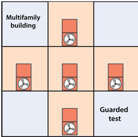
**Guarded test:** Attempts to measure the leakage to outdoors of a single dwelling unit. One blower door measures the units air leakage while other blower doors pressurize adjacent units to the same negative or positive pressure.
