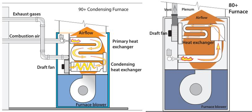
**90+ Gas furnace:** A 90+ furnace has a condensing heat exchanger and a stronger draft fan for pulling combustion gases through its more restrictive heat exchanger and establishing a strong positive draft.
