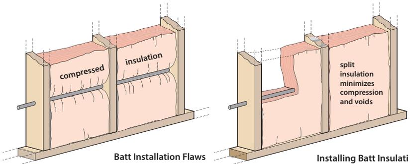
**Fiberglass batts, compressed by a cable:** This reduces the wall’s R-value by creating a void between the insulation and interior wallboard.
