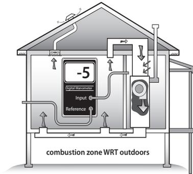
9. Calculate the net difference between the worst depressurization found from either #6 or #8 and the baseline pressure from #3. This is the worst-case depressurization.
