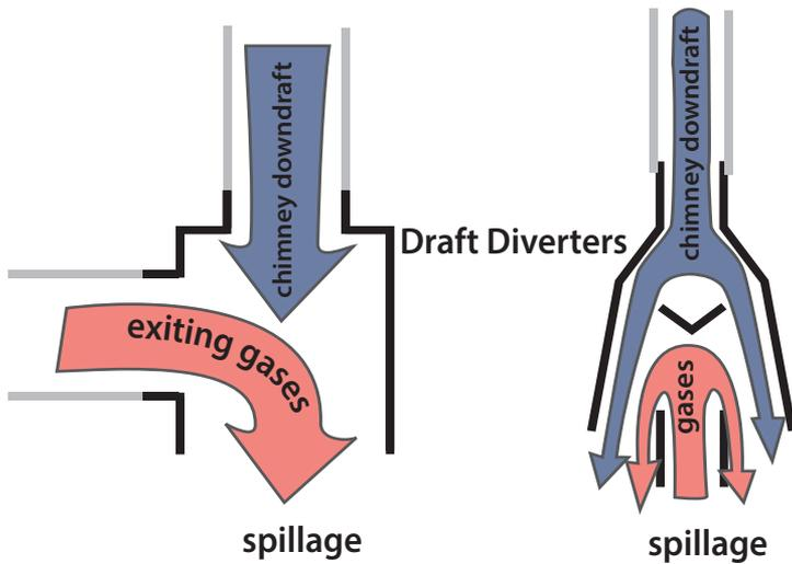
**Draft-diverter spillage:** Look for soot or corrosion near the draft diverter and also near the burner caused by spillage.
