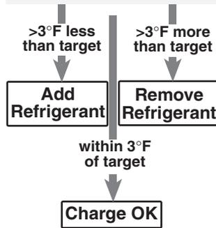
**Charge-checking:** Two methods help technicians judge whether the charge is correct. The remedy for incorrect charge is to either add or remove refrigerant.
