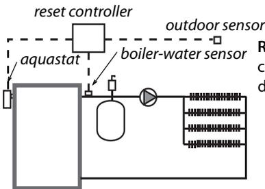
**Reset controller:** This control adjusts circulating-water temperature depending on the outdoor temperature.
