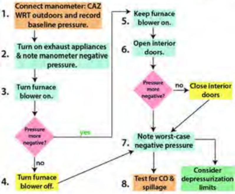
Spillage limits: 2 minutes warm chimney; 5 minutes cold chimney
