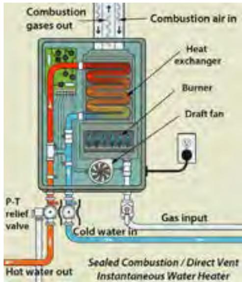
**Sealed-combustion on-demand water heater:** These water heaters have a small market share and save around one-third of energy used by the best storage water heaters.
