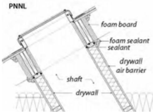
**Insulated and air sealed skylight:** The skylight shaft must be insulated and air sealed from the ceiling to the roof.
