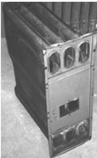
**Furnace heat exchangers:** Although no heat exchanger is completely airtight, it shouldn't leak enough to display the warning signs described here.
