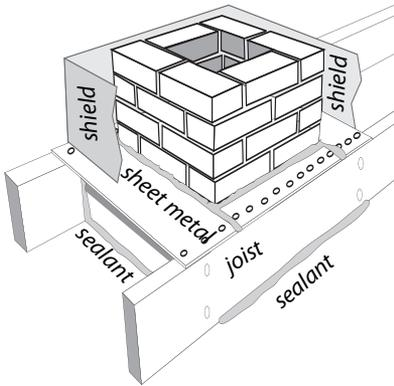
**Sealing around chimneys:** Chimneys require both an air seal and a shield if retrofit insulation is installed with air sealing.
