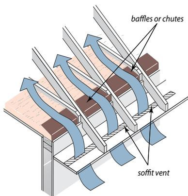
**Ventilation pathways:** Install baffles or chutes in every roof bay where soffit or eave venting exists.
