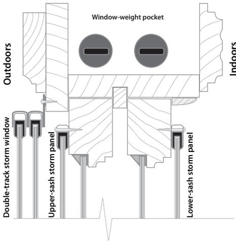
**Optimized double-hung window:** An exterior aluminum storm window plus storm window panels on the window sashes create triple glazing in this double-hung window.
