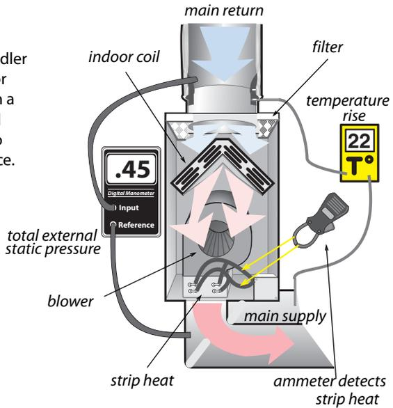
Heat pumps are also equipped with auxiliary electric resistance heat, called strip heat. The energy efficiency of a heat pump depends on how much of the heating load the compressor provides without using the strip heat.
