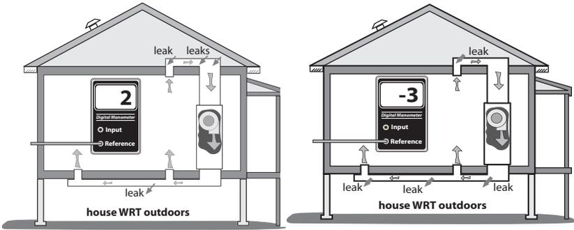
**Dominant return leaks:** When return leaks are larger than supply leaks, the house shows a positive pressure with reference to the outdoors.
