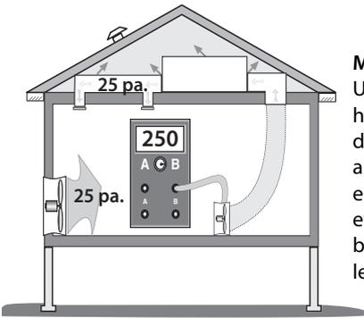
**Measuring duct leakage to outdoors:**
