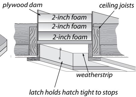
**Insulated attic hatch:** Building a dam prevents loose-fill insulation from falling down the hatchway. Foam insulation prevents the access hatch from being a thermal weakness. Install foam to achieve attic-insulation R-value of R-38. Foam can be glued together in layers.
