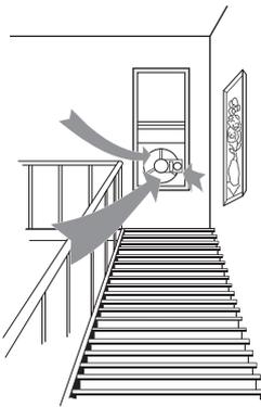
**Window fans:** Window fans circulate outdoor air when it is cooler than indoor air. The air circulation removes heat from the house.
