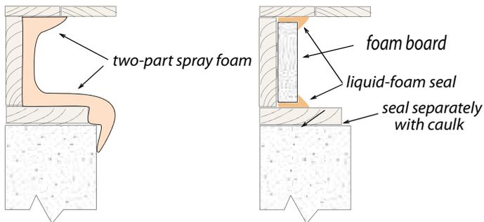
**Foam-insulated rim joists:** Installing foam insulation is the best way to insulate and air seal the rim joist.
