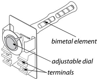
**Fan/limit control:** Turns the furnace blower on and off, according to temperature. Also turns the burner off if the heat exchanger gets too hot.
