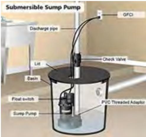
**Sump pump:** Pumps water out of a sump or basin where water collects in a basement or crawl space.
