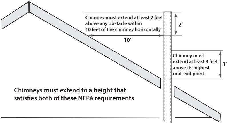
**Chimney terminations:** Should have vent caps and be given adequate clearance height from nearby building parts. These requirements are for both masonry chimneys and manufactured all-fuel chimneys.
