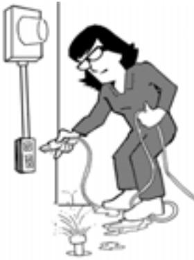
**Electrical safety:** Maintain cords in good condition. Use ground-fault-circuit interrupter (GFCI) cords for outlets in wet conditions.
