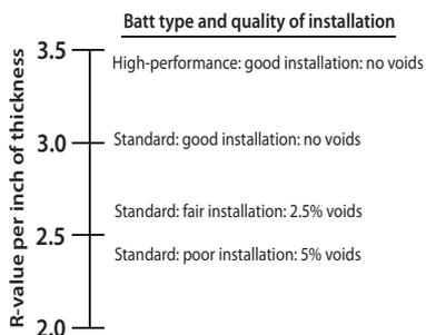
Installers must cut and fit batts very carefully. Batt s achieve their advertised R-value only when they are touching all six sides of the cavity it inhabits.
