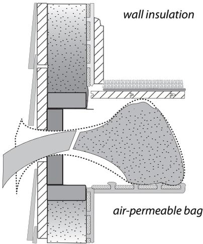
**Floor cavities:** Floor cavities are difficult to fill in platform-framed homes. Blow a plug of insulation into the floor cavity to insulate this uninsulated area.
