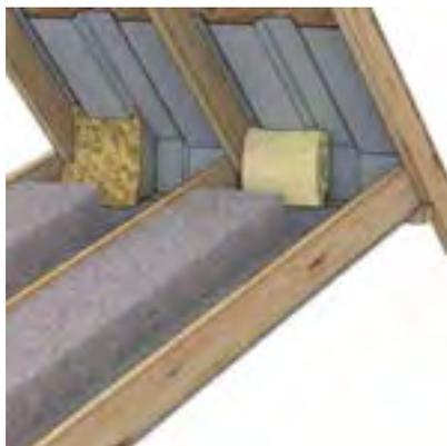
**Insulation at the eaves:** Stuff fibrous insulation into the eave area to maximize R-value. Use mechanical fasteners to attach the baffles to the framing.
