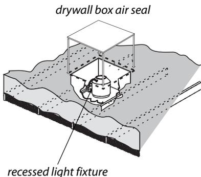
**Air seal and shield for non-IC can:** This drywall box is an insulation shield and air seal, but allows the fixture some air circulation for cooling.
