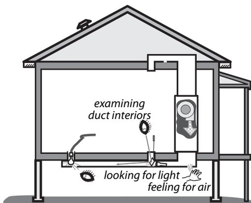
1. Use the air handler blower to pressurize supply ducts. Closing the dampers on supply registers temporarily or partially blocking the register with pieces of carpet, magazines, or any object that won't be blown off by the register's airflow increases the duct pressure and make duct leaks easier to find. Dampening your hand makes
