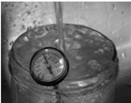
**Setting hot-water temperature:** Getting the temperature correct can take a few measurements and re-adjustments.
