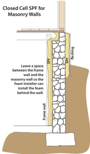
**2-part foam sprayed on rubble masonry:** Installers insulate rubble masonry walls on the interior or exterior with sprayed plastic foam. On the interior, they cover the foam with drywall.
