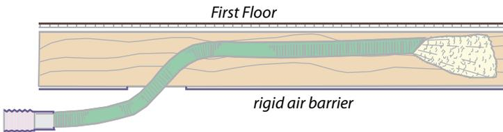
**Blowing floor cavity:** Uninsulated floor cavities can be blown with fiberglass or rock wool insulation, using a fill tube.
