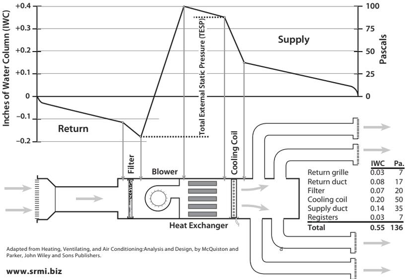
**Visualizing TESP:** The blower creates a suction at its inlet and a positive pressure at its outlet. As the distance between the measurement and blower increase, pressure decreases because of the system's lower resistance.
