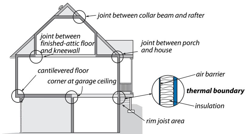
**Air leaks at the thermal boundary:** The air barrier and insulation, which should be adjacent to one another, are located at the thermal boundary. The insulation and the air barrier are often discontinuous at corners and transitions.
