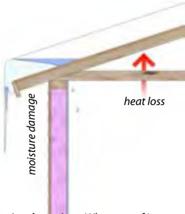
**Ice damming:** When a roof is unventilated, the home's heat loss warms the roof deck melting snow. The water re-freezes at the eaves and causes moisture damage.
