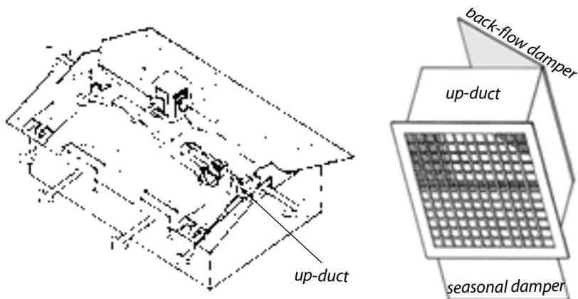
**Air circulation:** Outdoor air is sucked through the evaporative cooler and blown into the home pushing house air out of the partially open windows. Some dwellings with evaporative coolers employ up-ducts instead of open windows for security concerns.
