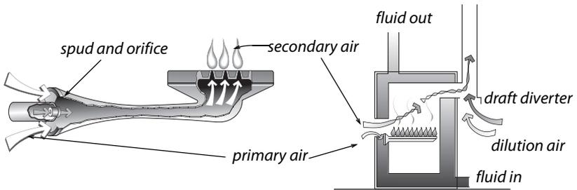
**Natural-draft, open combustion gas burners:** Combustion air comes from the indoors in open combustion appliances. These burners use the heat of the flame to pull combustion air into the burner. Dilution air, entering at the draft diverter, prevents overfire draft from becoming excessive.
