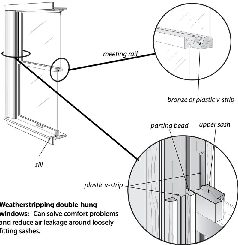
**Weatherstripping double-hung windows:** Can solve comfort problems and reduce air leakage around loosely fitting sashes.
