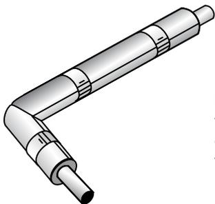
**Properly installed pipe insulation:** Must be the right size for the pipe, must completely cover the pipe, including bends, and must be fastened tightly to the pipe.
