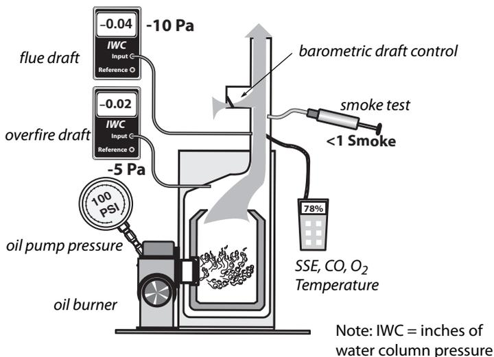
**Measuring oil-burner performance:** Measuring oil-burning performance requires, a manometer, flue-gas analyzer, smoke tester, and pressure gauge.
