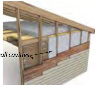
**Balloon framed gable:** Studs extend above the ceiling allowing convection from the attic.
