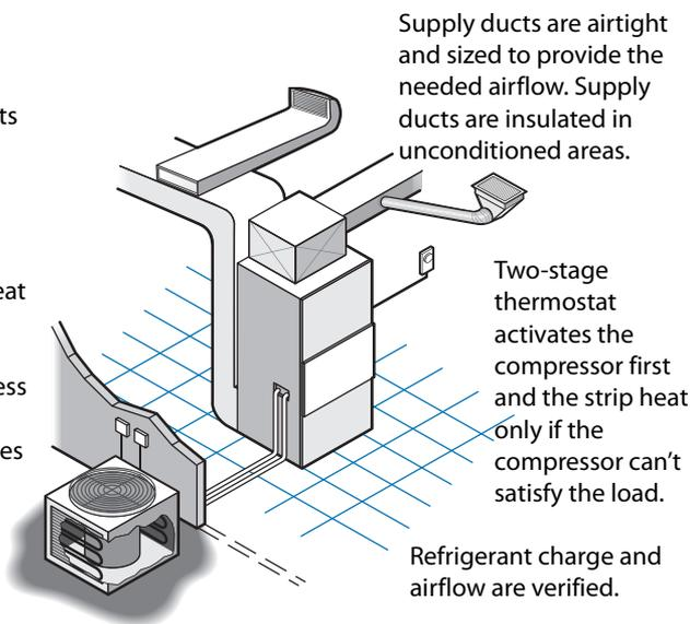
Supply ducts are airtight and sized to provide the needed airflow. Supply ducts are insulated in unconditioned areas.
