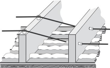
**Knob-and-tube wiring:** Replace obsolete and worn wiring during energy retrofit work so that workers can insulate building cavities sufficiently.
