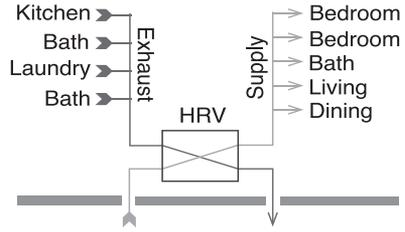
Balanced ventilation systems can improve the air quality and comfort of a building, but they require a high standard of care. Testing and commissioning are vital during both the initial installation and periodic service calls.
