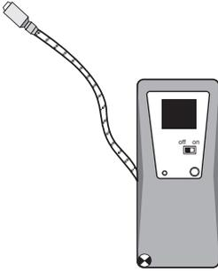
**Gas sniffer:** Use this device to detect the presence of combustible gases around fittings.
