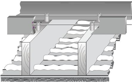
**Shielding knob and tube:** If you can't decommission knob-and-tube wiring, you may construct a dam to shield the wiring from insulation.
