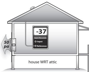
**House-to-attic pressure:** This commonly used measurement is convenient because it requires only one hose.
