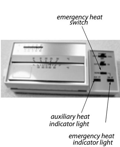
**Heat pump thermostat:** These should have two indicator lights, one for auxiliary heat and one for emergency heat.
