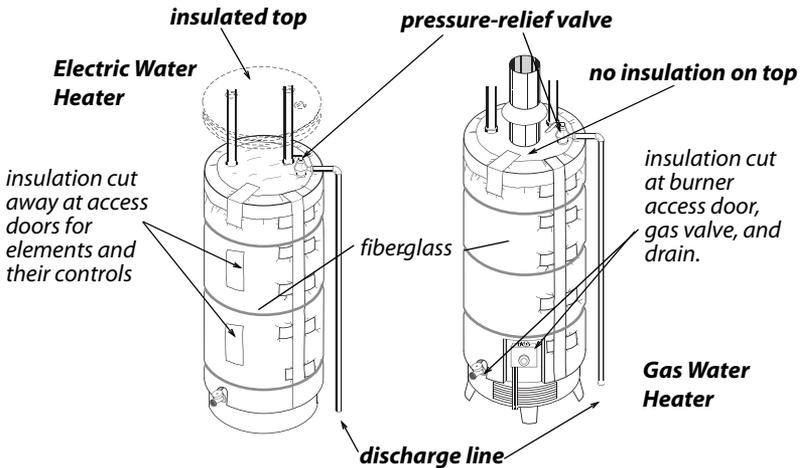
**Water heater insulation:** Insulation should be installed carefully so it doesn't interfere with the burner, elements, draft diverter, FVIR combustion intake, or pressure relief valve and discharge line.
