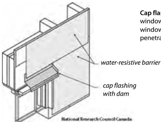
**Cap flashing:** Cap flashing at the window's head protects the window from rain water penetration.
