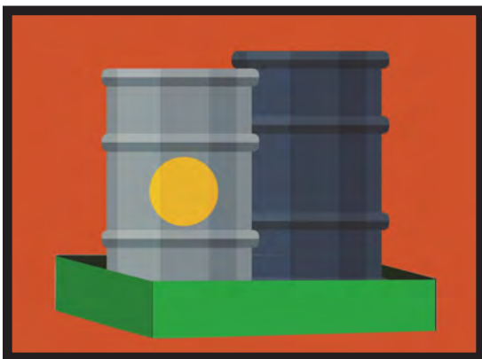
Store liquids in secondary containment and always label the containers
