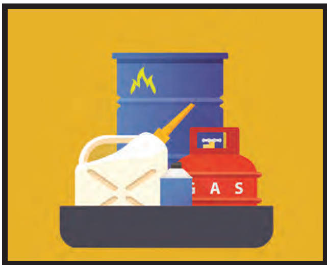
Materials that could spill should be stored in secondary containment.
