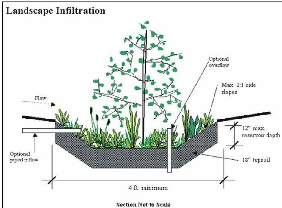
Typical Bioretention Cross-section
