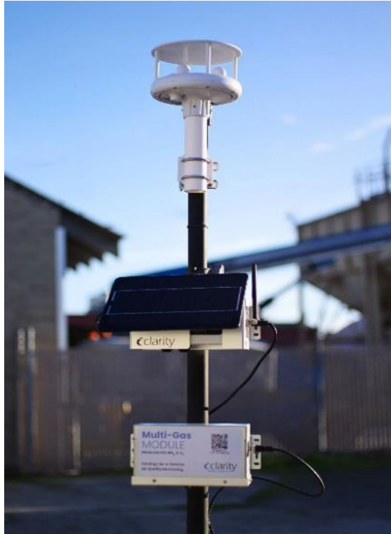
Clarity Node sensor measures PM_{2.5} , NO_2 , Ozone, and meteorological data
