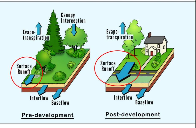
Surface runoff is minimal in an undeveloped site, but dominates the water balance at a highly impervious site.
